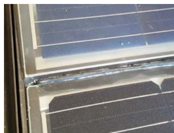
Sealing compound is to be discharged at the edges of the module
